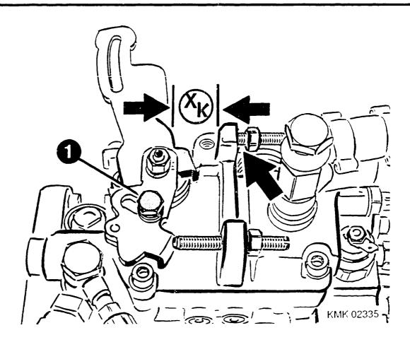
ADJUSTING CONTROL-LEVER POSITION "XK"
